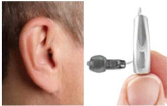
Barely visible when worn, the RIC style is an instrument in which the receiver, or speaker, is inside the ear canal. Thin electrical wires are used instead of a plastic acoustical tube, reducing distortion. RIC hearing aids provide a comfortable, open fit. For mild to moderate hearing loss.
